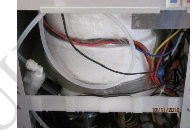
Be sure the fittings are tight in the solenoid water valve. It does not matter what position the fittings are in. The solenoid water valve just sits any where beside the tank or where ever there is room and the hoses can reach it. The valve can be mounted using 2 short screws but it is not necessary.
