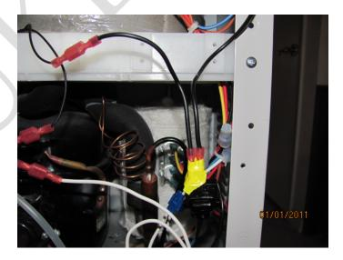
Next you can either let the switch dangle in the back or mount it. Once the kit is installed, you'll only need to turn off the bottle free conversion when you go on vacation or to work on it. I'd recommend unplugging it when ever you work on it.
