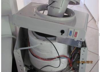
Drill a 5/16" hole through the insulation and metal tank. Slide a 12" piece of hose through the hole and put a <sup>1</sup>/<sub>4</sub> inch Union Elbow on the end in the tank.
