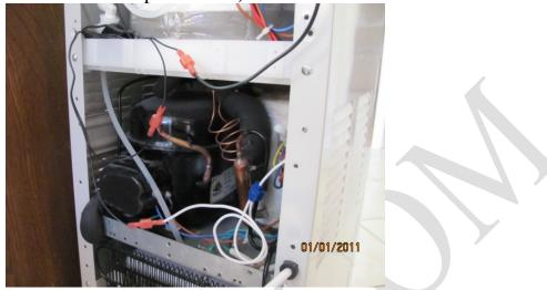
Connect the other side of the water float switch to the white wire. Connect the other end of the white wire to the white wire in the cooler using the splice connector. Make sure you connect the white wire to the white wire close to where it comes out of power cord.
