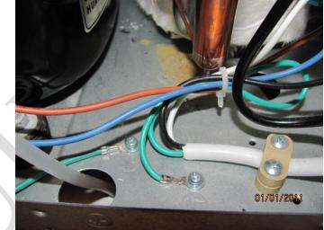
You may need to put a multimeter on the switch to determine which side is hot and which side is off when the switch is off. On my cooler, the black wire is connected to a red wire that is connected to the hot and cold switches so I knew that the other wire connected to the switch was off when the switch was off.
