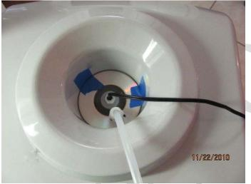
Pick a spot near the back of the cooler next to the rim. Drill a 3/8 inch hole. You may need to expand it a bit to get the wire connectors through or use a 1/2" bit.
