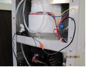
Connect the other wire from the solenoid to one wire of the water float switch (one of the wires coming from the water float switch in the plastic disk).
