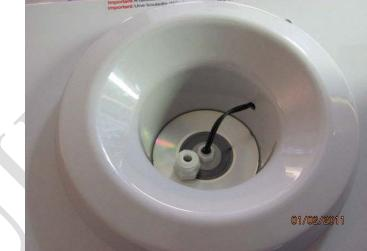
Loosen the rim and feed the water float switch wire through the 2 holes. One side of the water level switch connects to the solenoid valve and the other wire connects to the white wire. Please see the instructions above. You can remove the water inlet fitting from the disk.
