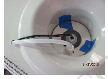
Choose which fittings you want in the valve. I left them out incase you wanted to use the straight fitting in the disk next to the water float switch. If you use the alternate installation you can use a straight push on fitting on both sides of the water valve. Be sure to put some teflon tape on the fitting's threads.
