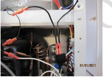
Wrap a piece of tape around the switch connectors just to be sure they do not come in contact with any other metal. I used the insulated crimp connectors so we really don't have to worry about this. Better to be safe.
