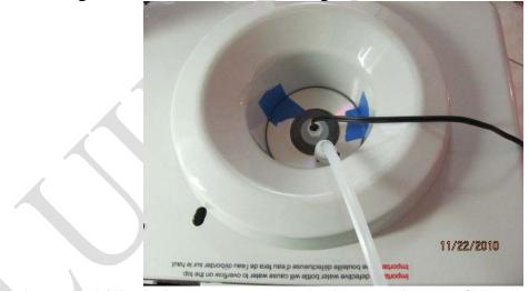
You don't have to drill a hole. You can run the hose and water float switch wire to the back and duct tape them to the tank or some where in the back. I've given this some thought, you don't really need any tools to install this device except maybe a pair of pliers.
